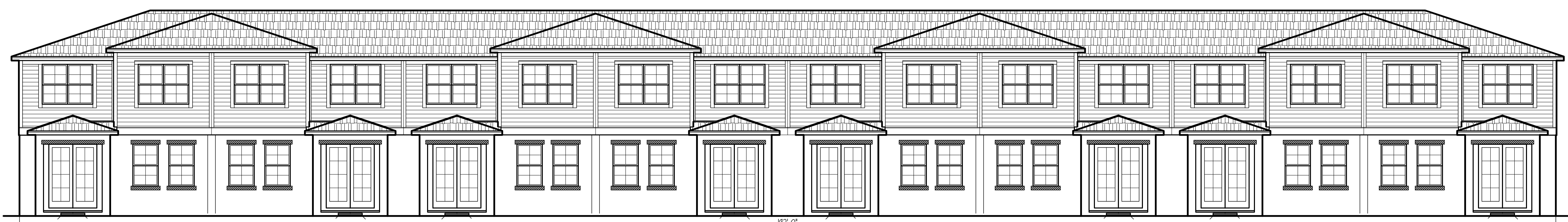
BLDG TYPE 3 - FRONT ELEVATION 1/4"=1'-0"
