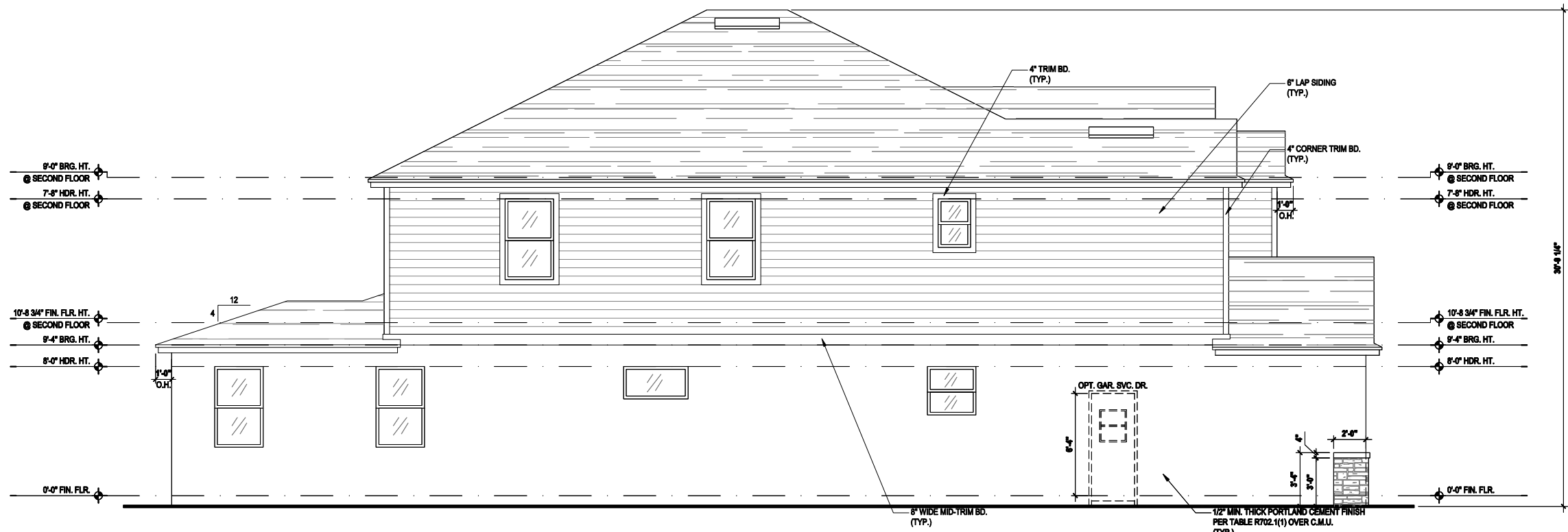
Left Elevation "C" w/ Siding (Opt. Extended Bonus Rm.) SCALE 1/8" = 1'-0" (11x17) 1/4" = 1'-0" (22x34)
