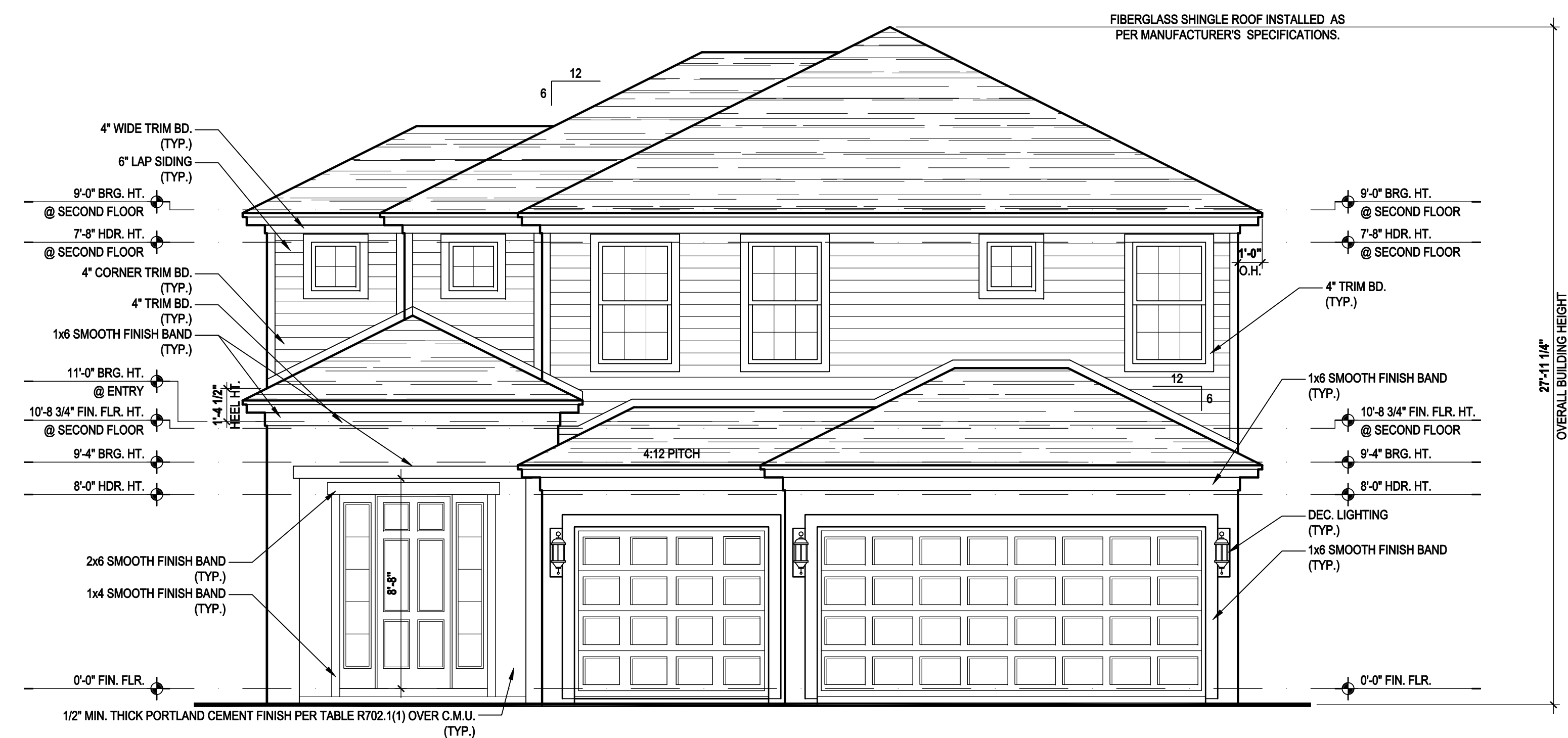
Front Elevation "A" (Opt. Bed 5-Bath w/ Ext. Cov. Lanai) SCALE 1/8" = 1'-0" (11x17) 1/4" = 1'-0" (22x34)
