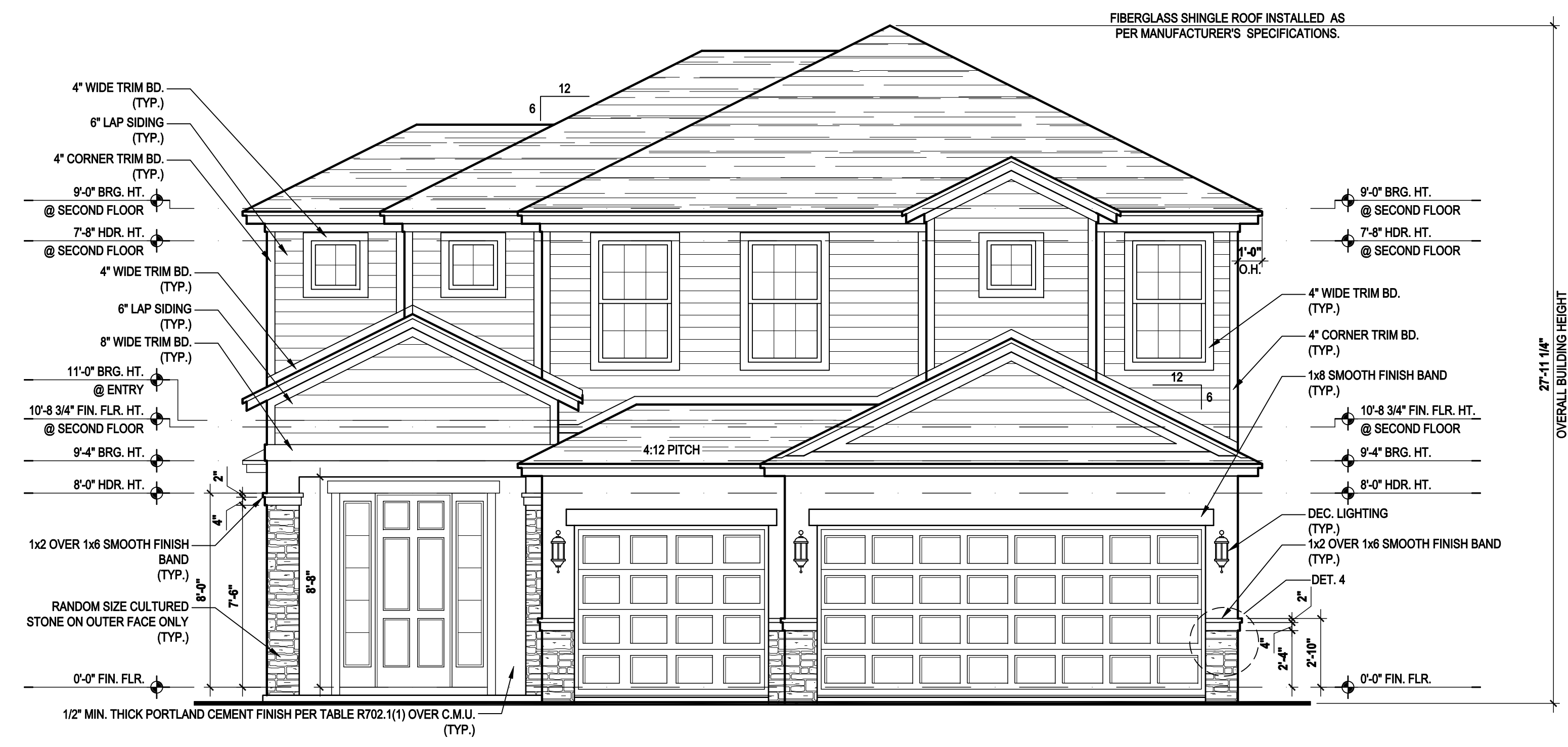
Front Elevation "C" (Opt. Bed 5-Bath w/ Cov. Lanai) SCALE: 1/8" = 1'-0" (11x17) 1/4" = 1'-0" (22x34)
