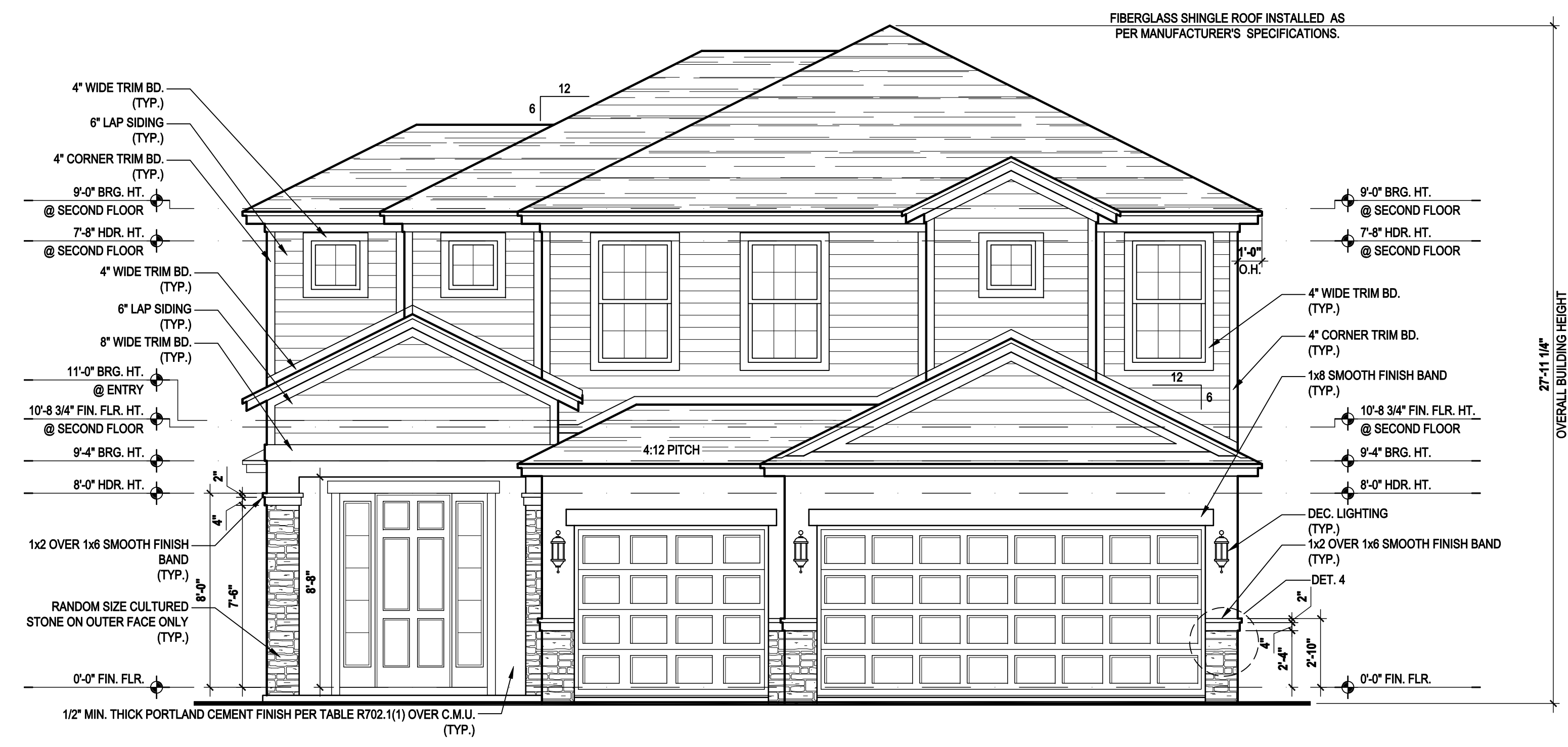
Front Elevation "C" (Opt. Bed 5-Bath w/ Full Cov. Lanai) SCALE: 1/8" = 1'-0" (11x17) 1/4" = 1'-0" (22x34)
