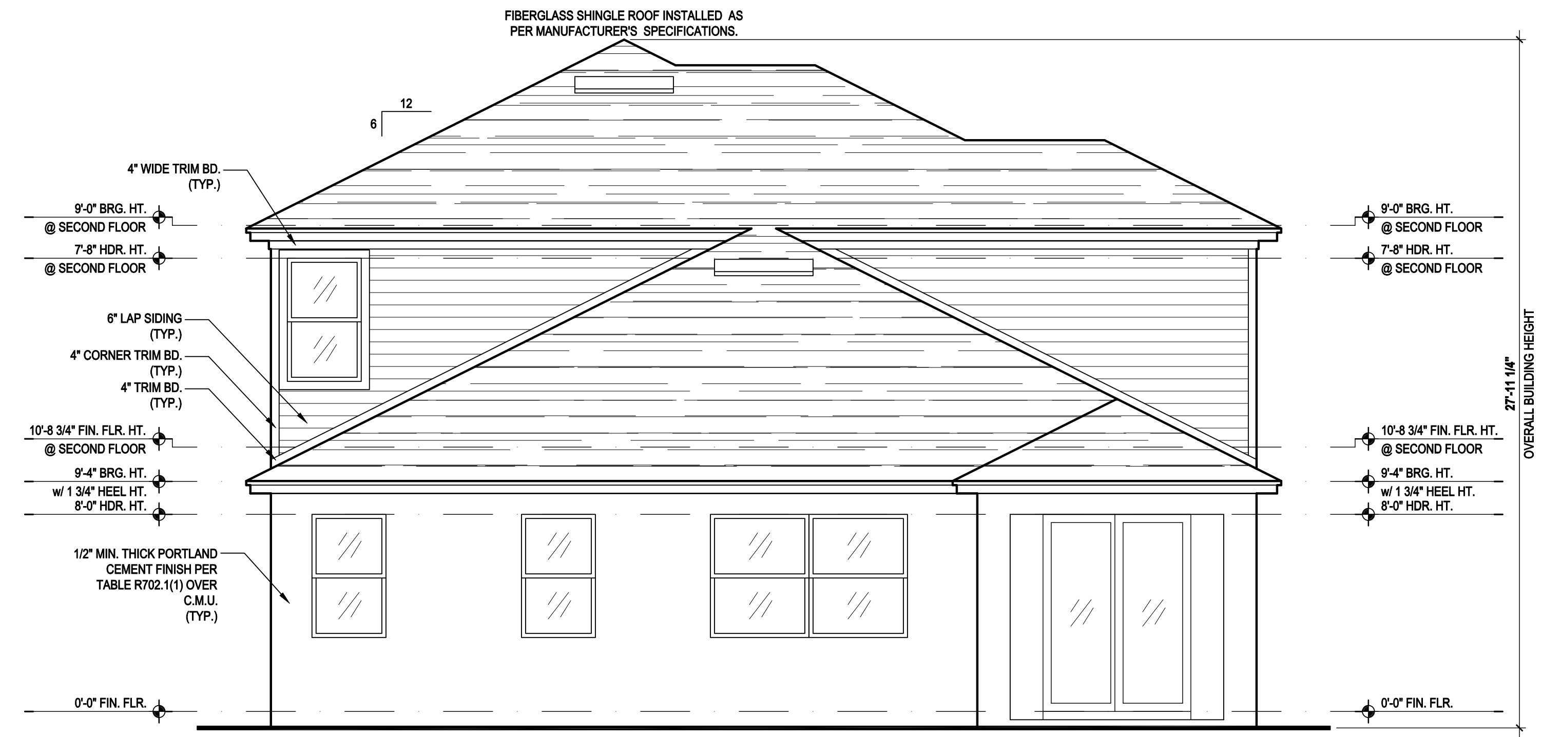
Front Elevation "A" (Opt. Bed 5-Bath w/ Cov. Lanai) SCALE 1/8" = 1'-0" (11x17) 1/4" = 1'-0" (22x34)
