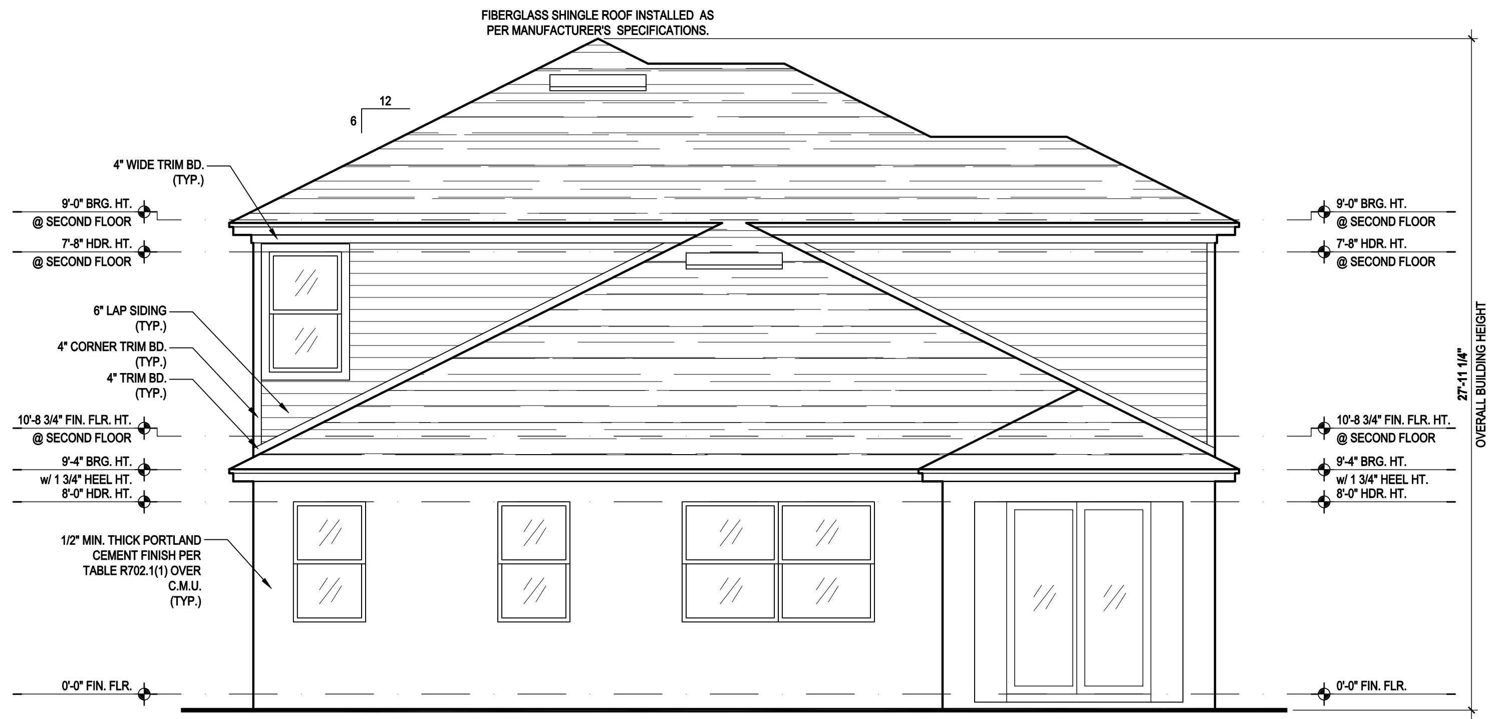
Front Elevation "B" (Opt. Bed 5-Bath w/ Cov. Lanai) SCALE 1/8" = 1'-0" (11x17) 1/4" = 1'-0" (22x34)
