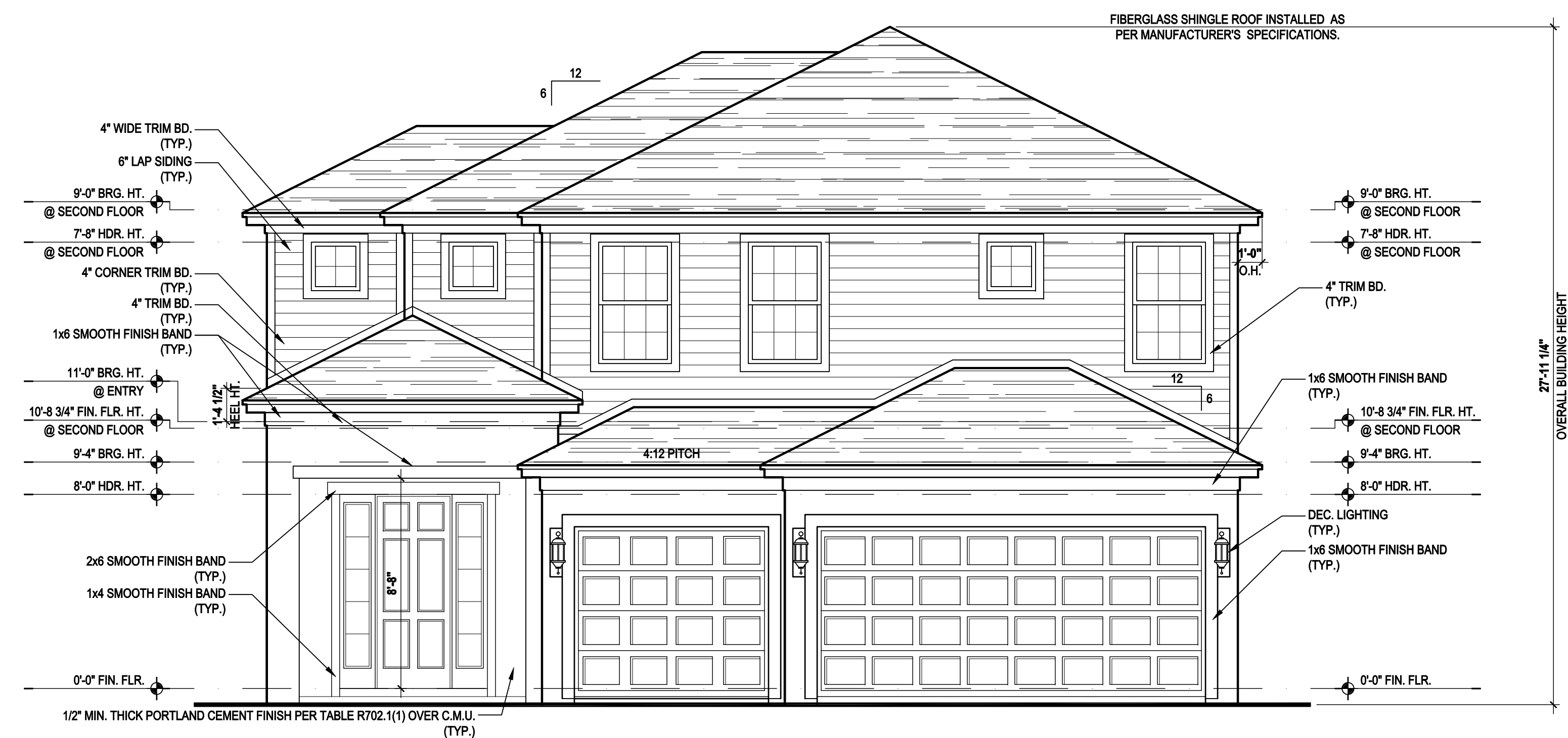
Front Elevation "A" (Opt. Bed 5-Bath w/ Full Cov. Lanai) SCALE 1/8" = 1'-0" (11x17) 1/4" = 1'-0" (22x34)
