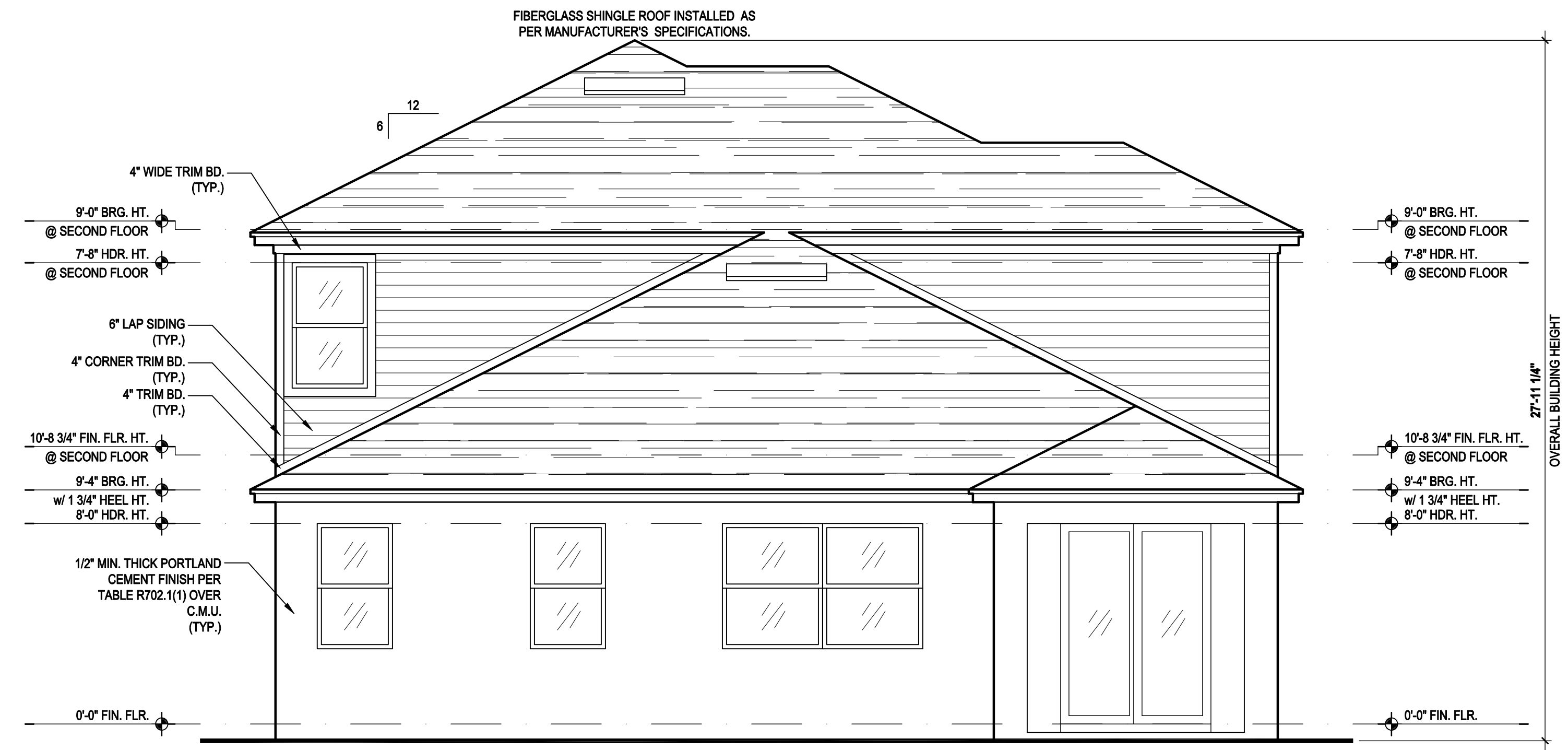
Front Elevation "C" (Opt. Bed 5-Bath w/ Cov. Lanai) SCALE: 1/8" = 1'-0" (11x17) 1/4" = 1'-0" (22x34)
