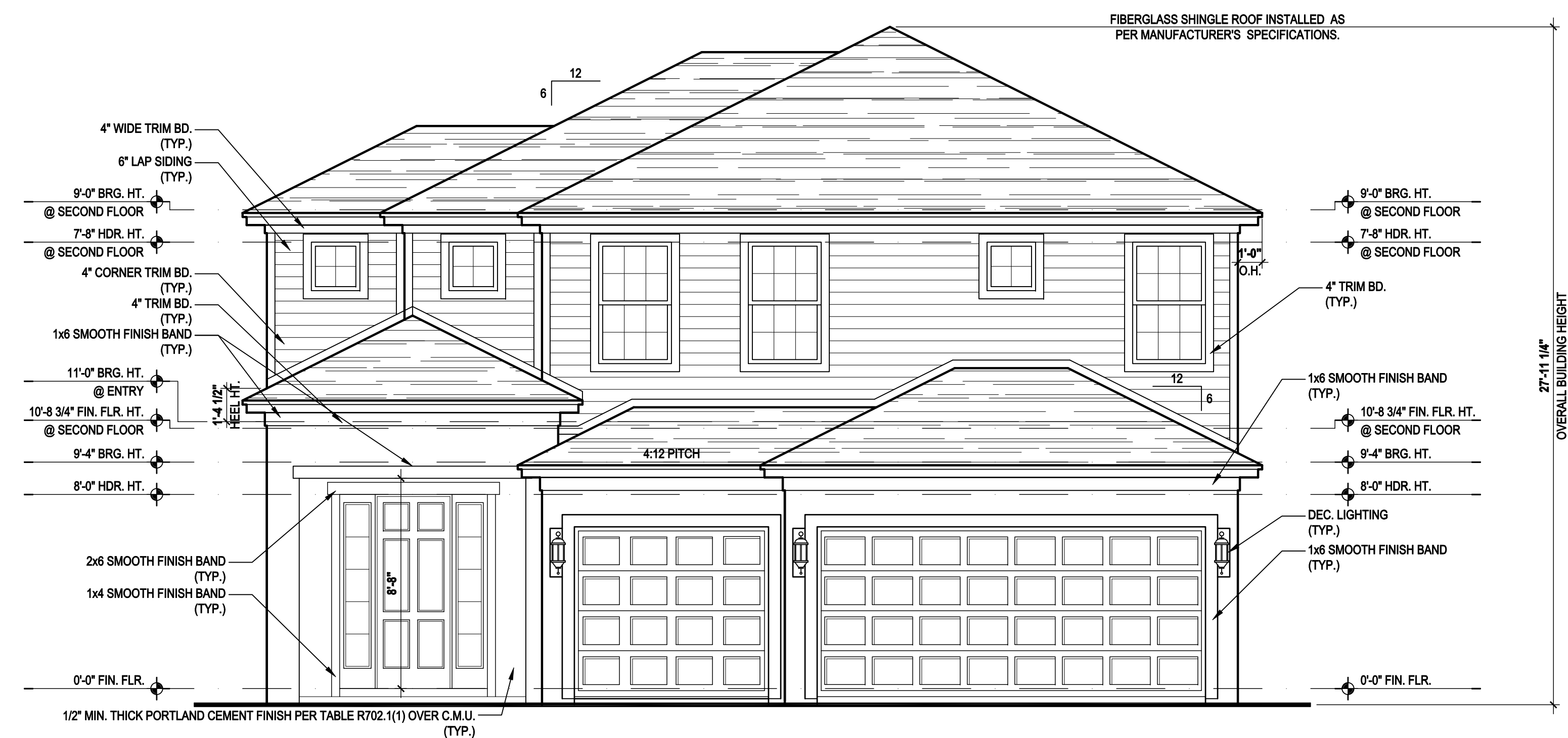
Front Elevation "A" (Opt. Bed 5-Bath w/ Cov. Lanai) SCALE 1/8" = 1'-0" (11x17) 1/4" = 1'-0" (22x34)
