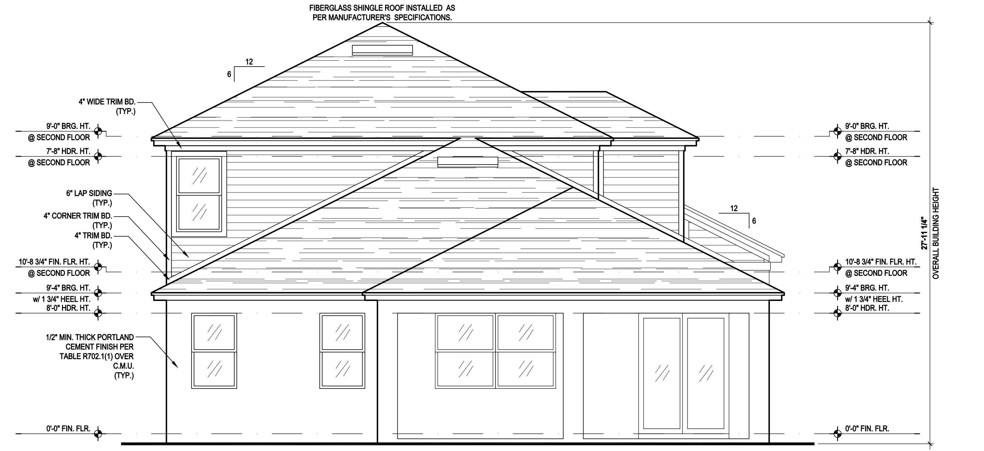
Front Elevation "A" (Opt. Bath 3 w/ Ext. Cov. Lanai) SCALE 1/8" = 1'-0" (11x17) 1/4" = 1'-0" (22x34)
