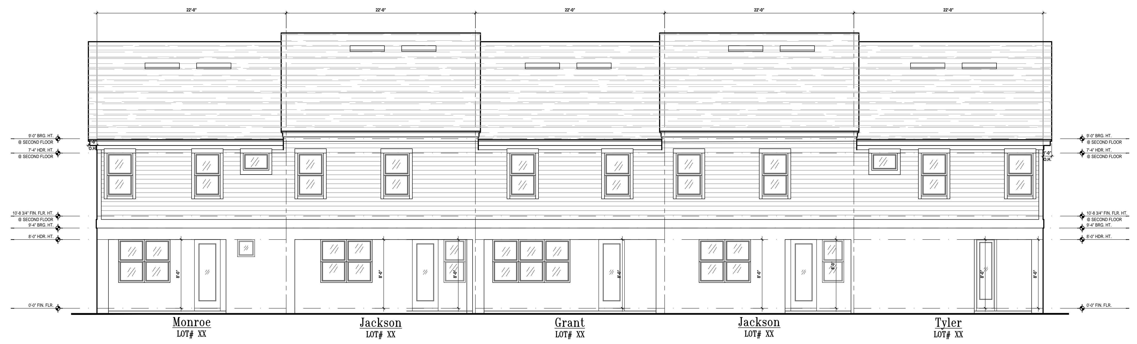
Rear Elevation: Courtyard SCALE: 3/16" = 1'-0"
