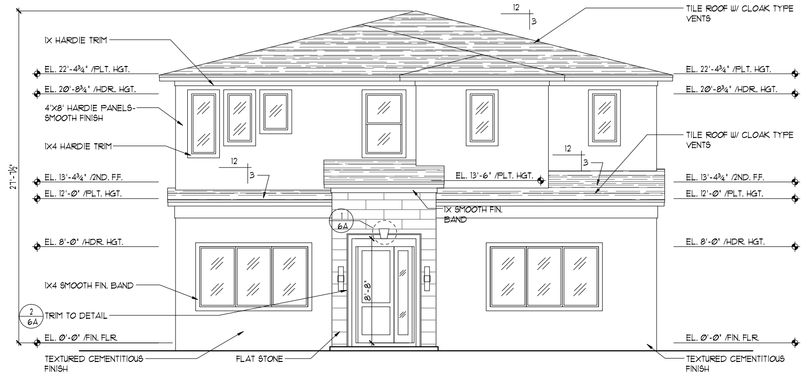
FRONT ELEVATION "A" 1/8"=1'-0" (11X17) 1/4"=1'-0" (22X34)
